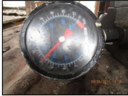
Fig.4 Pressure gauge applied for checking of prestress level applied (Courtesy:- M/s R & M International Pvt Ltd)
